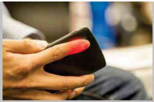
HemaApp measures hemoglobin levels and screens for anemia non-invasively by illuminating the patient's finger with a smartphone's camera flash. Dennis Wise/University of Washington
